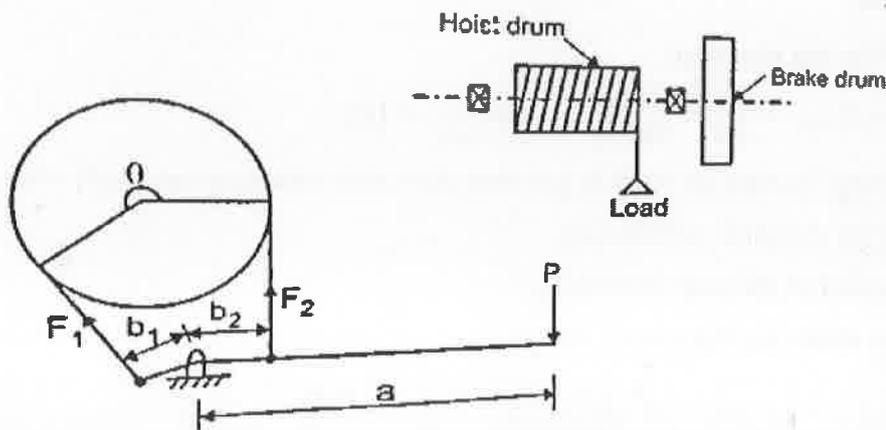
Braking torque,  $T_b = \text{load to be lifted} \times \text{barrel radius} = 20000 \times 0.3 = 2000 \text{ N} - \text{m}$
